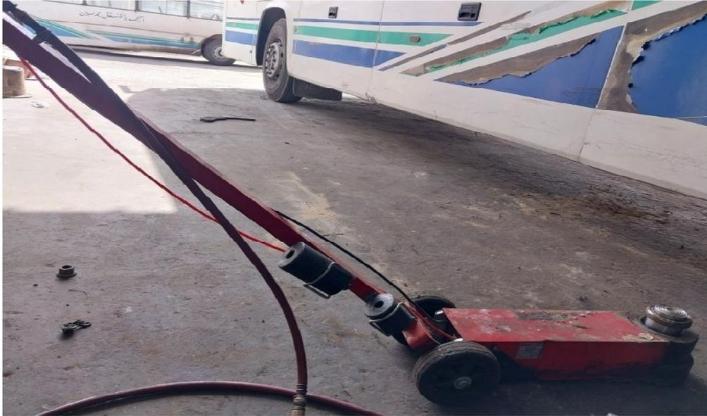
Figure 34: cric hydraulique
