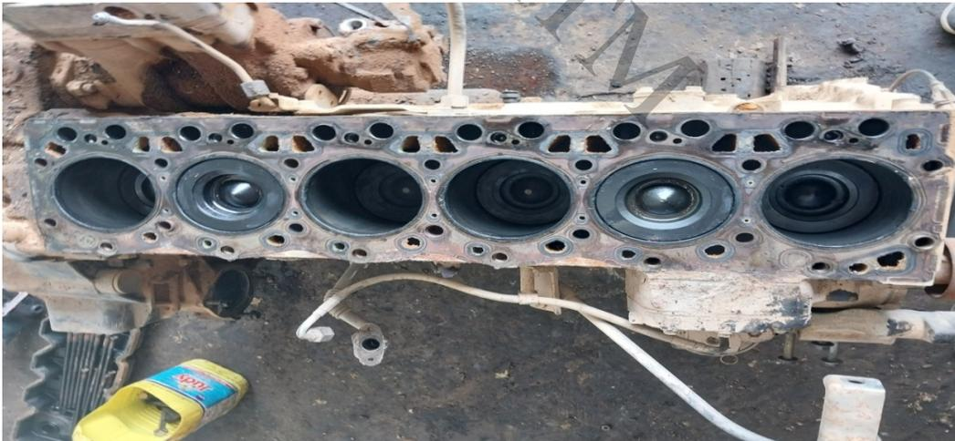
Figure 5: Bloc cylindre
