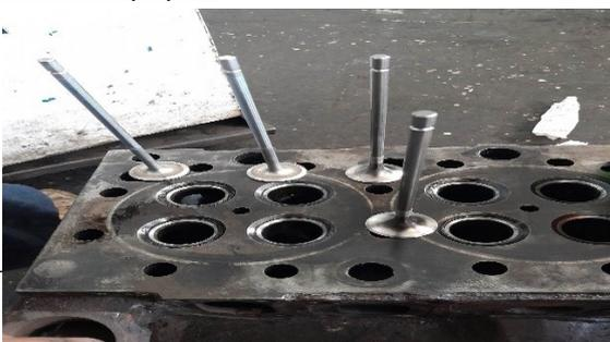
Figure 15 : soupape
